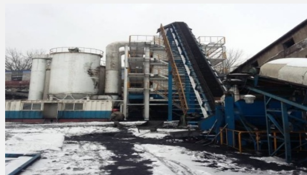
60-0mm Wet Coal Separation (1.0 Mtpa, Yushan Coal Mine)
